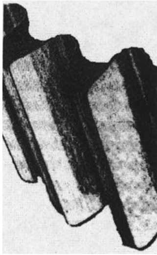
Figure 10-2 Normal wear pattern.
