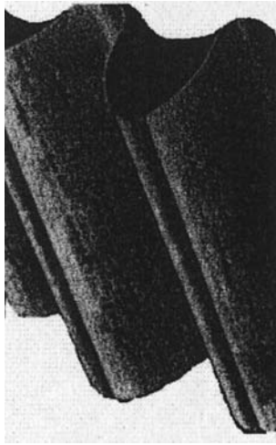
Figure 10-4 Pattern caused by corrosive attack on gear teeth.
