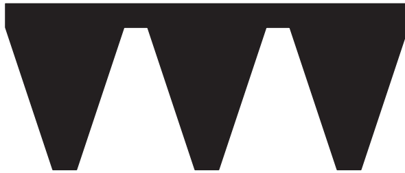
Figure 23.5 Joined belt (VX type)
