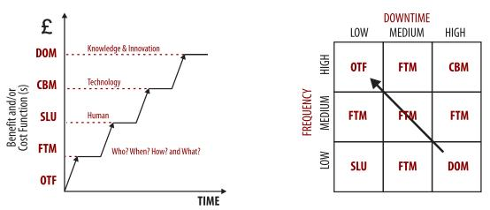
OTF:Operate to Failure SLU:Skill Level Upgrade CBM:Condition Based Maintenance FTM:Fixed Time Maintenance DOM:Design Out Maintenance
