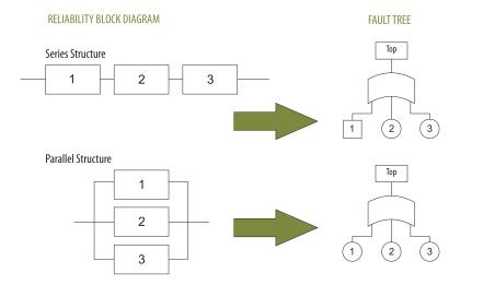
Figure 3: Fault Tree Analysis: Connection to reliability
